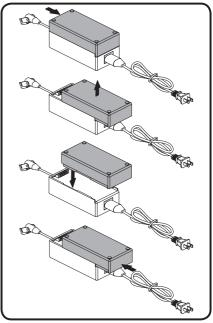
Figure B Lithium-Ion Battery Replacement
